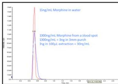
Figure 4: Morphine extracted from a 1000ng/mL DBS spot compared to a solution of morphine in water
