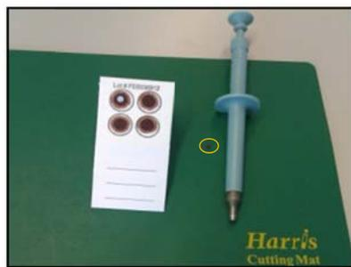
Figure 3: Blood samples (20µL) were spotted onto Whatman DMPK B DBS cards and dried. 3mm punches were then taken for extraction
